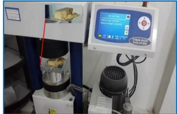
**Fig. 8.** Brick sample (TS1-1) in the compression machine shows cracking at 25.6 KN/m<sup>2</sup> of the peak load.
