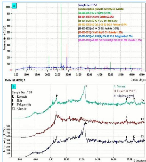
**Fig. 3.** XRD diffractograms of claystone sample TS7-1; **A)** Bulk sample, **B)** oriented clay fraction in different treatment stages.
