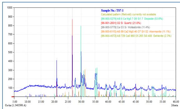
**Fig. 9.** XRD diffractograms of claystone (brick sample TS7-1) burned to 950°C.
