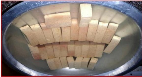
**Fig. 5.** Brick samples immerse in water during the water absorption test.
