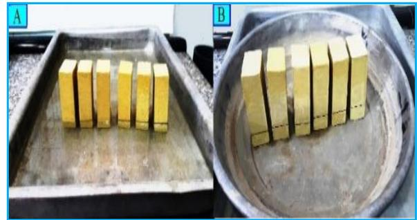
**Fig. 6.** Efflorescence test for some brick samples A-during immersed in water, B-after dried from water.
