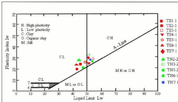
**Fig. 4.** The plasticity diagram shows the results of plasticity limits for claystone samples.
