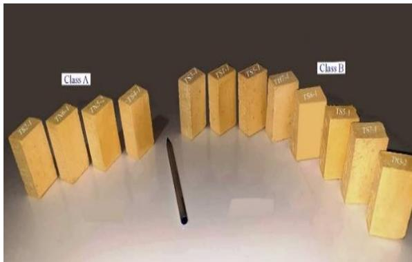
**Fig. 7.** Claystone brick samples belonging to categories A and B.
