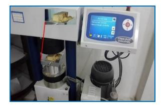
Fig. 8. Brick sample (TS1-1) in the compression machine shows cracking at  $25.6 \text{ KN/m}^2$  of the peak load.
