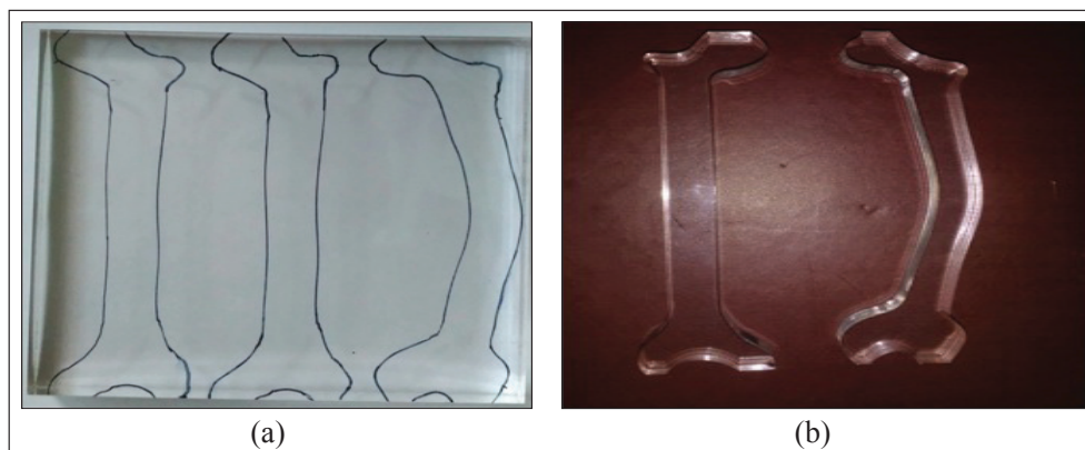
Fig. 2. femur model (a) marked in acrylic sheet, (b) cut piece of femur model
