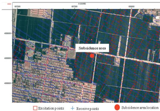
Fig. 10. Site layout of excitation and receiving points near collapse area.
