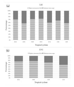
**Fig. 5.** The proportions of astronomical tide and storm surge in total water level in storm cases at LSI (a) and LYG (b)
