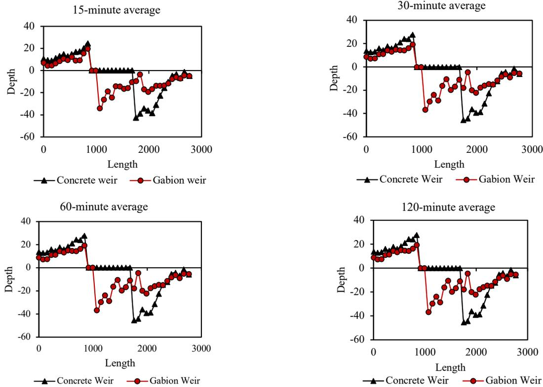
**Fig. 7.** Longitudinal profiles of sedimentation and scouring for both types of weir models at different durations
