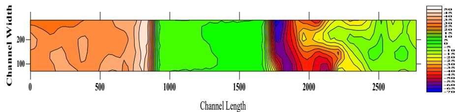
**Fig. 6(b).** Contour map showing the affected area around Concrete weir for 120-minute duration
