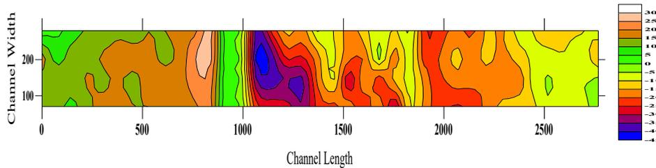
**Fig. 5(a).** Contour map showing the affected area around gabion weir for 60-minute duration
