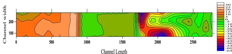
**Fig. 3(b).** Contour map showing the affected area around concrete weir for 15-minute duration
