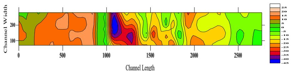
**Fig. 4(a).** Contour map showing the affected area around gabion weir for 30-minute duration
