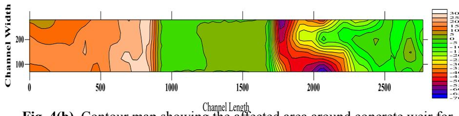
**Fig. 4(b).** Contour map showing the affected area around concrete weir for 30-minute duration
