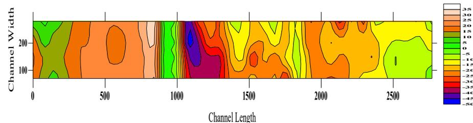
**Fig. 6(a).** Contour map showing the affected area around gabion weir for 120-minute duration
