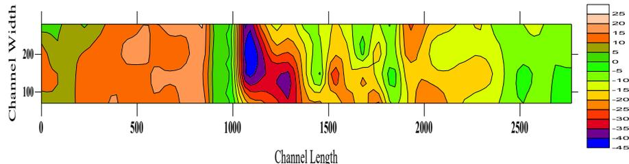
**Fig. 3(a).** Contour map showing the affected area around gabion weir for 15-minute duration
