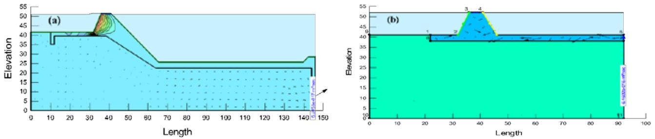
Fig. 8. Seepage analysis results for the (a) concrete and (b) gabion weir using Seep/W software
