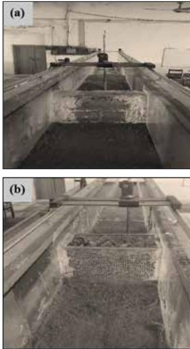
**Fig. 2.** Laboratory model for (a) concrete weir and (b) gabion weir
