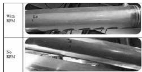
**Fig. 19.** The effect of pipe rotation on hole cleaning (size 0.2 mm)
