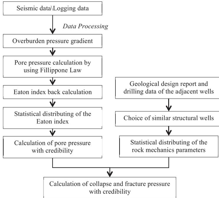
**Fig. 1.** Flowchart for calculating formation pressure with credibility
