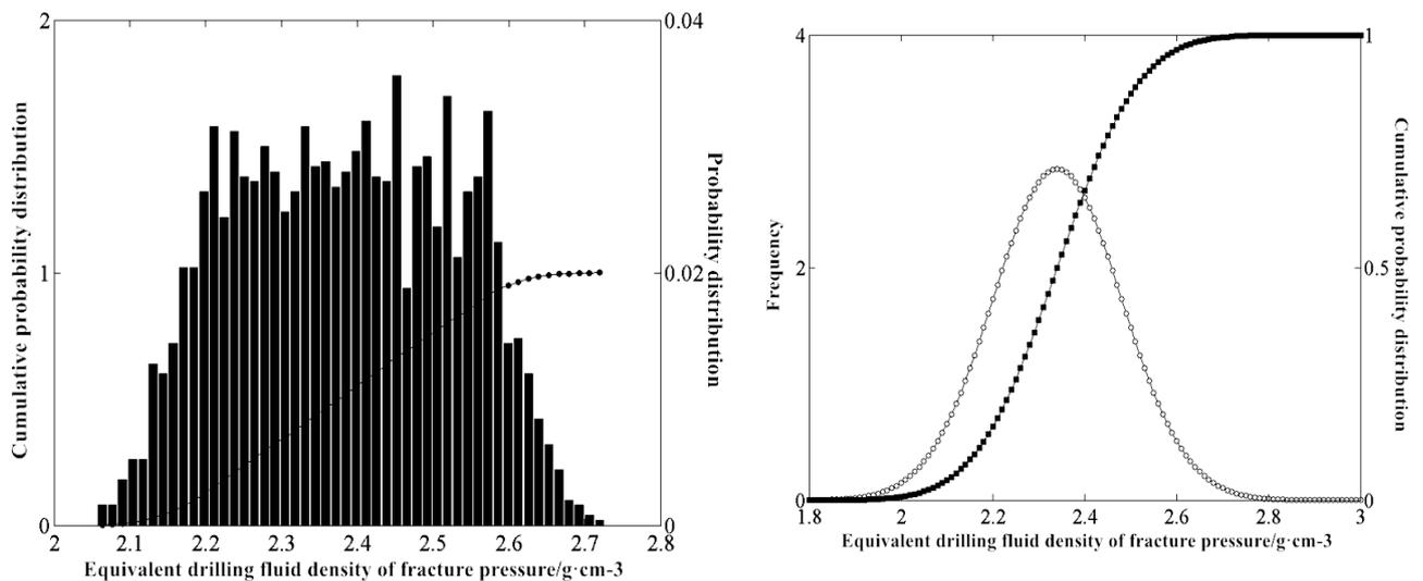
Fig. 5. Probability distribution of fracture pressure
