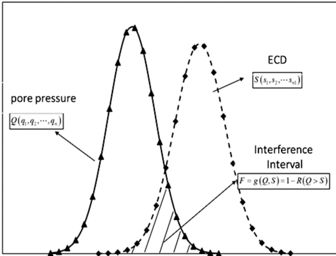
Fig. 2. Schematic diagram of well kick
