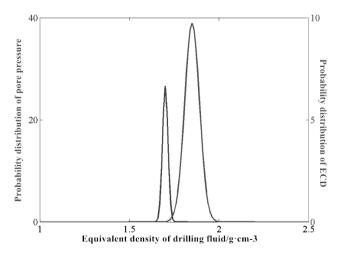
Fig. 7. Schematic diagram of well kick risk evaluation
