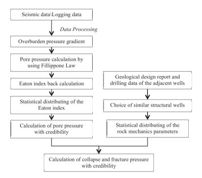
Fig. 1. Flowchart for calculating formation pressure with credibility
