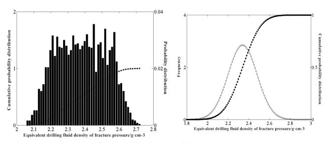
Fig. 5. Probability distribution of fracture pressure
