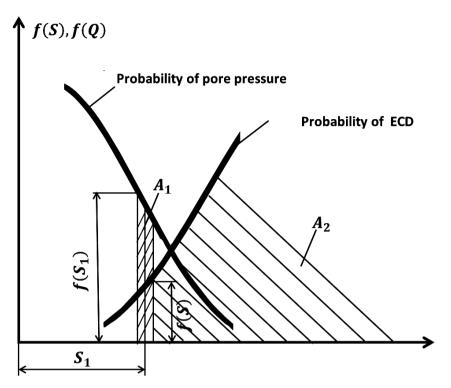
Fig. 3. Interference between pore pressure and ECD
