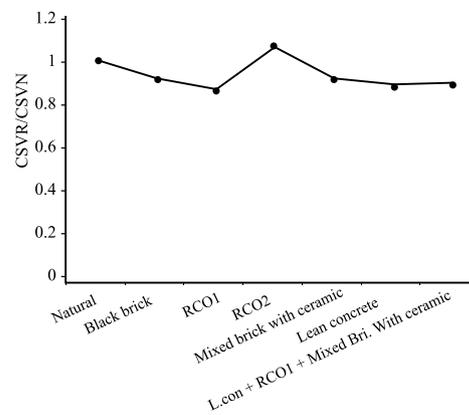
**Fig. 9.** A comparison between the compression strength values (CSVN) for recycled concrete samples and natural sample (CSVN).
