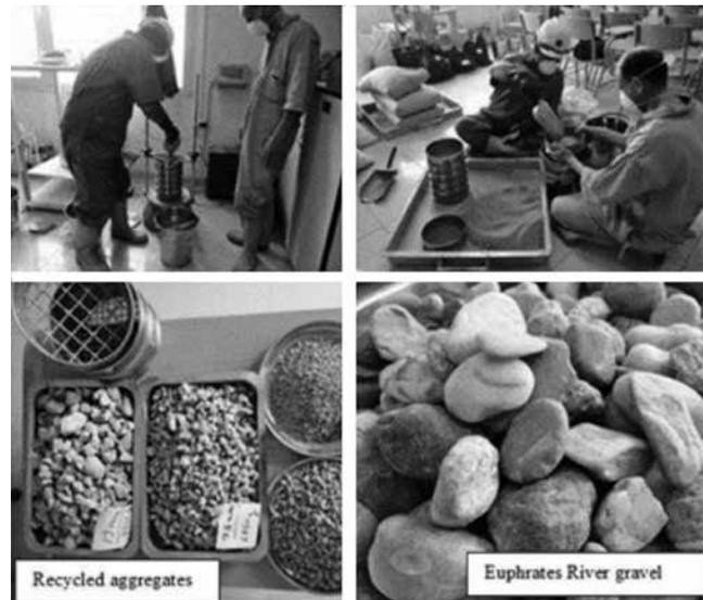
**Fig. 5.** Part of sieving process in the laboratory
