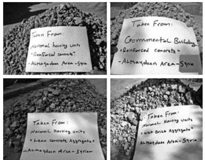
**Fig. 3.** Some types of recycled aggregate after hand crushing.
