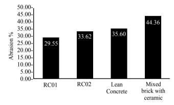
Fig. 6. Results of abrasion test for recycled aggregates
