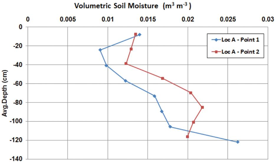
Fig. 5. Volumetric sub-surface soil moisture (22 Jan 2012)
