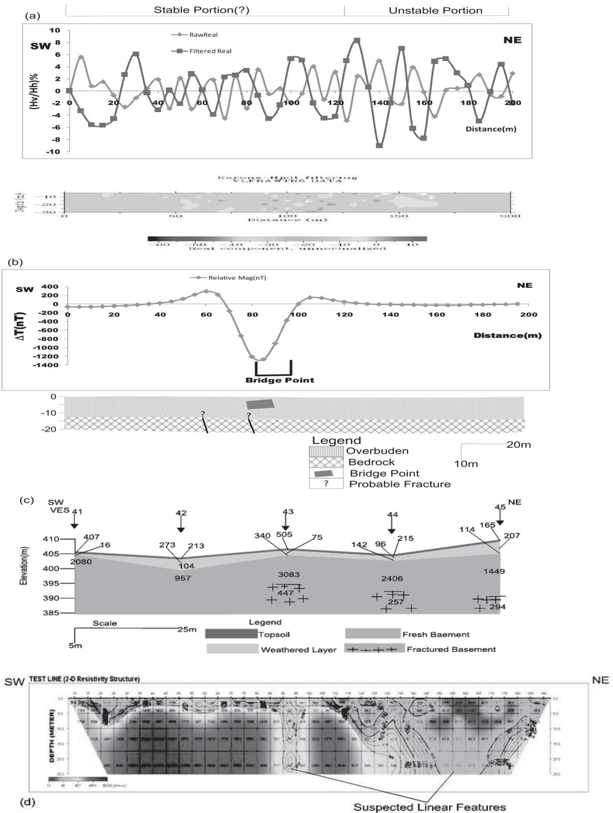
Fig. 11. (a) VLF-EM profile & corresponding section, (b) Magnetic profile & corresponding section, (C) Geoelectric section, and (d) 2-D Resistivity structure along traverse 6 at locality 3
