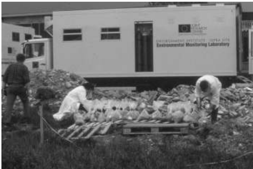
Fig. 2. The AMAL on-site in Waldau in 1993, with sample processing proceeding prior to analyses in the truck.
