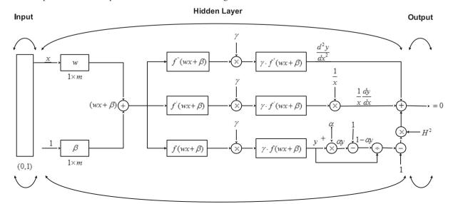
Fig. 2. Architecture of neural network model for EHD
