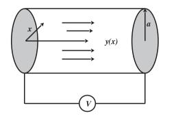
Fig. 1. Ion-drag flow in a circular cylindrical conduit
