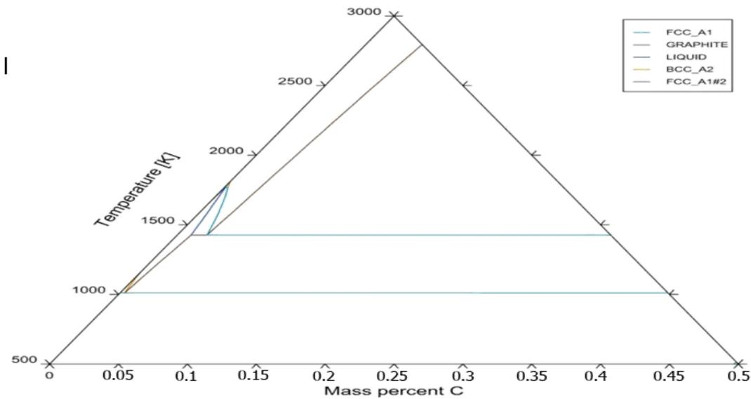
**Fig. 2.** Phase analysis section of the Ni rich solubility in the Fe-C system. Graphite phase is found highest molar volume in Ni-rich section for better solubility of Ni.
