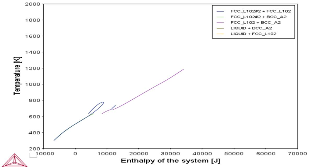
Fig. 6. Enthalpy of the region Ni doped at annealing of 1900K. Ni-rich section increases the entropy of BCC Phase of alloying at that Coupled Region shows still stability.
