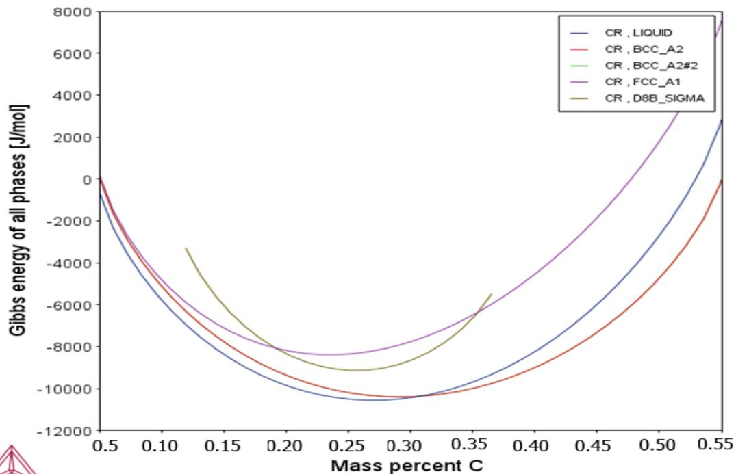
**Fig. 3.** Gibbs free energy of region Cr doped. The less Gibb energy value at 1900K shows Less Solubility of Cr-rich section.
