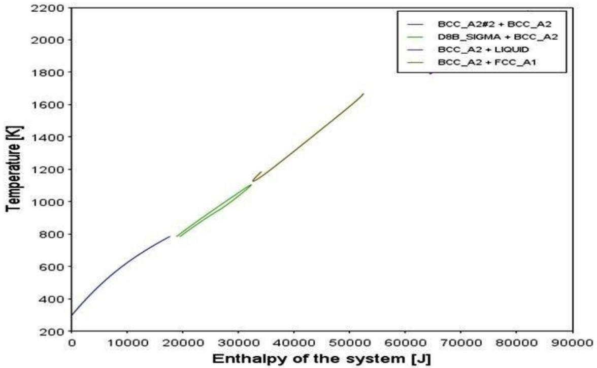
Fig. 5. Enthalpy formation of the region Cr doped at annealing of 1900K.
