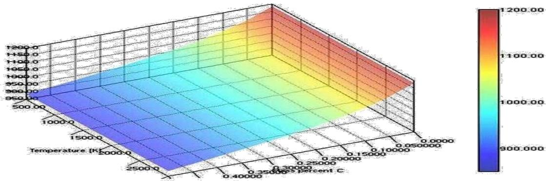
Fig. 7. T-zero analysis profile of Ni doped region at elevated temperature ranges.
