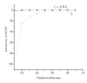
Fig. 7. MTTF sensitivity as a function of input parameters
