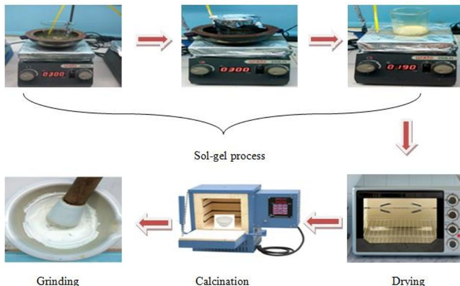
**Fig.1:** Sol-gel synthesis process of CaZnAl<sub>2</sub>O<sub>4</sub> nanoparticles.
