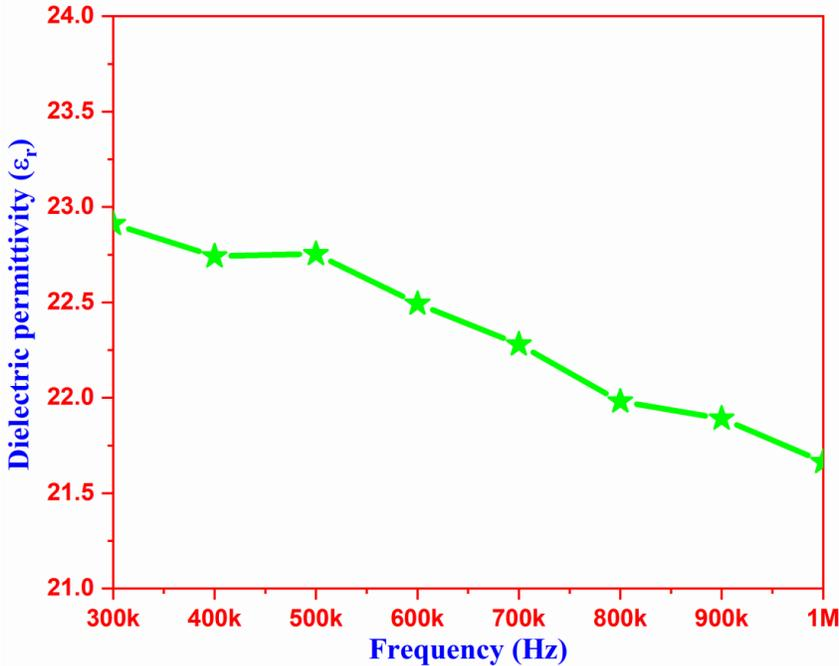
Fig.5: Dielectric permittivity of  $\text{CaZnAl}_2\text{O}_4$  ceramic nanoparticles.
