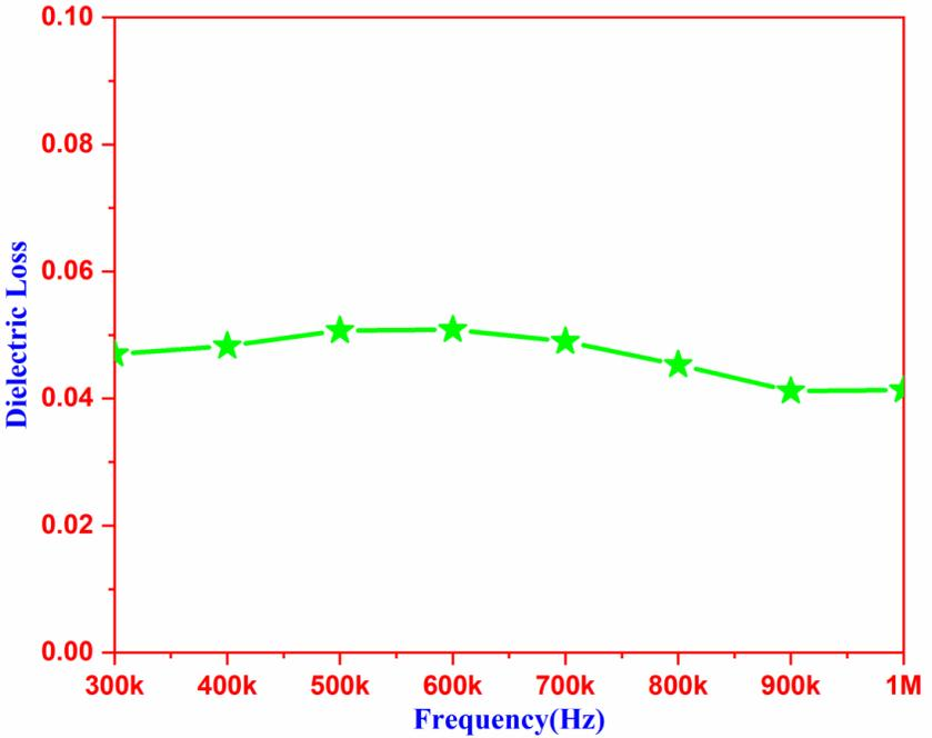
Fig.6: Dielectric loss of  $\text{CaZnAl}_2\text{O}_4$  ceramic nanoparticles.
