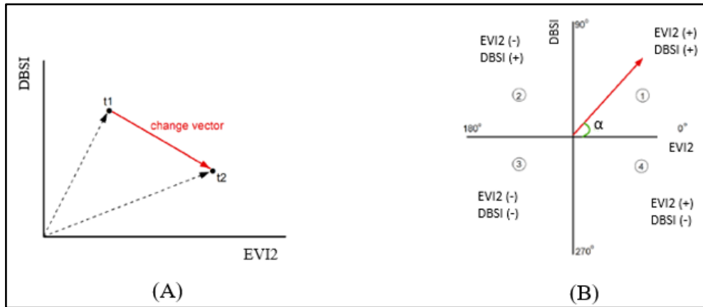
Fig. 3. The change vector analysis for space of EVI2-DBSI, (A) the magnitude of change and (B) the direction of change.
