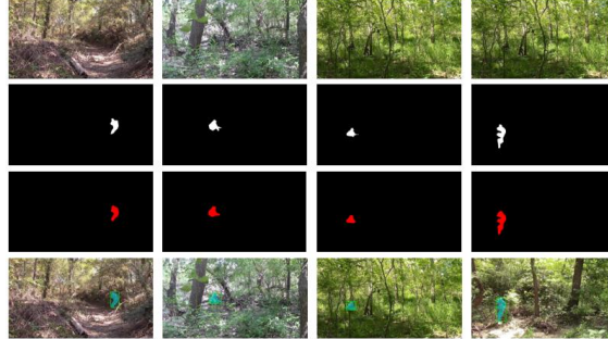
Fig. 5. Some examples of target detection results of our proposed approach. Image (row 1), GT (row 2), labeled image from our segmentation mask (row 3), and final detection (row 4).
