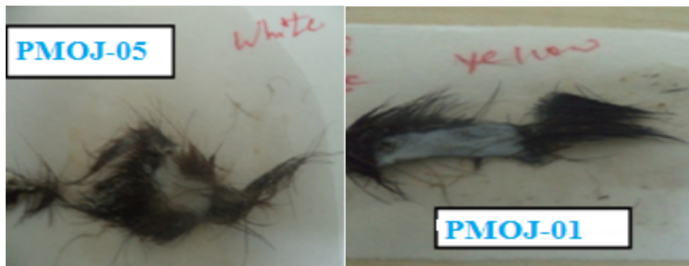
Fig. 10. De-hairing effect PMOJ-01( Pseudomonas aeruginosa ) enzyme and PMOJ-05 ( Bacillus subtilis )enzyme after 12 hours incubation
