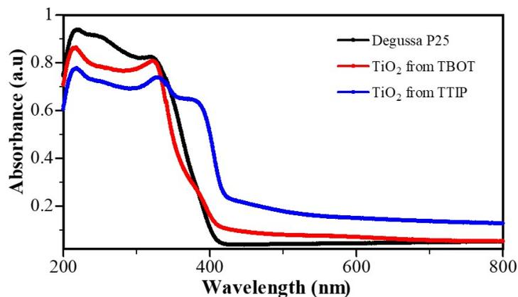
Fig. 2. Photocatalysts absorbtion in range 200-800 nm.
