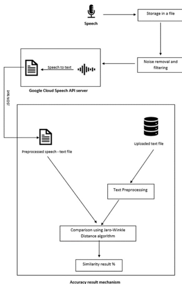
**Fig. 2.** The mechanism of the Samee'a system
