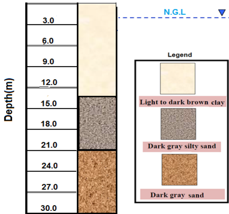
Fig. 2. The borehole section shows the soil profile and groundwater level in the study area (Al-Ebdaa Company, 2015).
